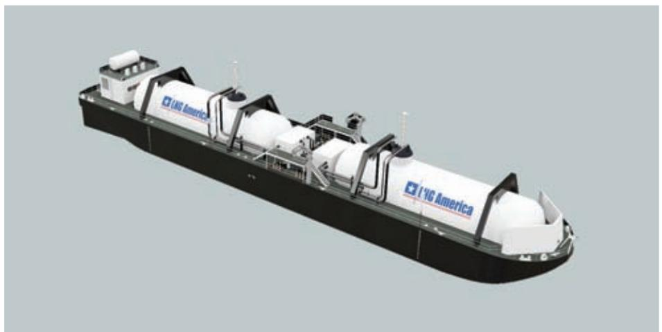
**The barge will be fitted with an IMO Type ‘C’ independent tank containment system.**
